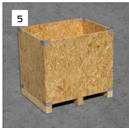
5 Fit the BeA VTT connectors at the top
