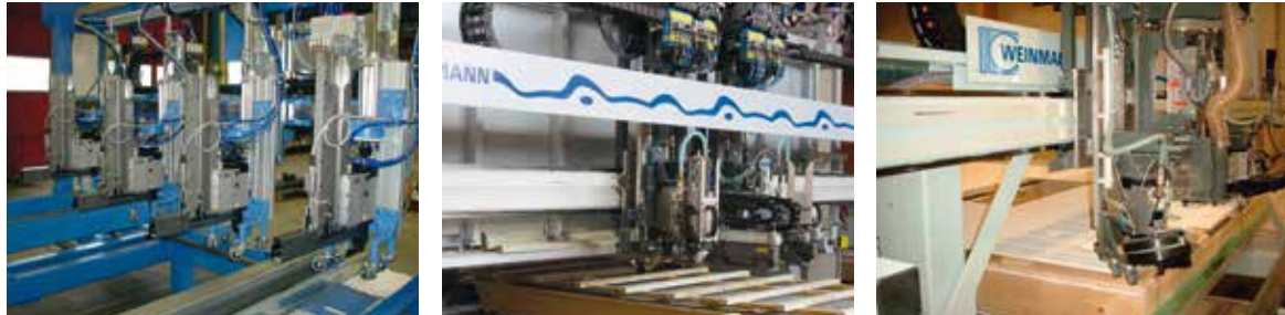
Stapling station integrated in production line
