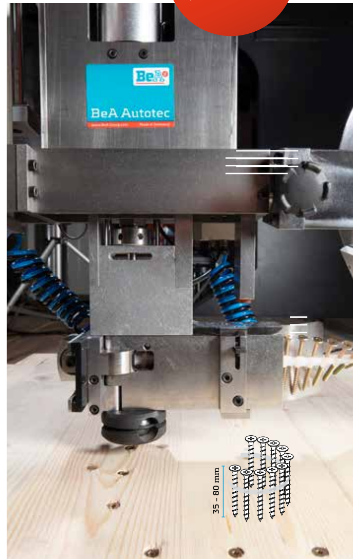
Jumbo coil: Magazine capacity 700 Screws
